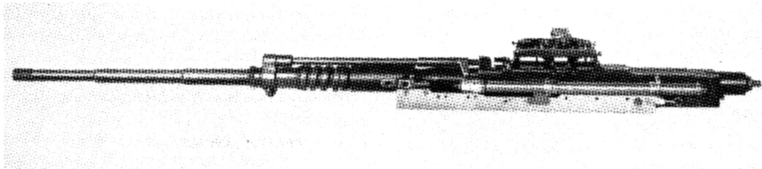
Figure 1-38. 20-mm Gun Mechanism Mk 16 Mod 0.
