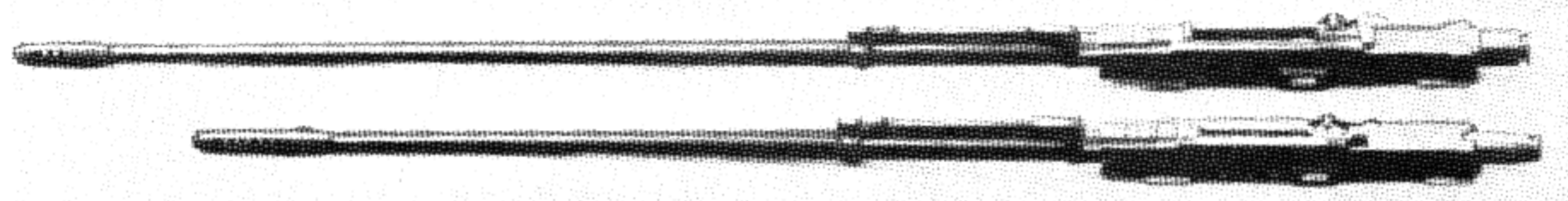
Figure 20-21. The basic 20-mm Hispano-Suiza Type 820 Gun (above) and the basic 20-mm Hispano-Suiza Type 804 Gun.
