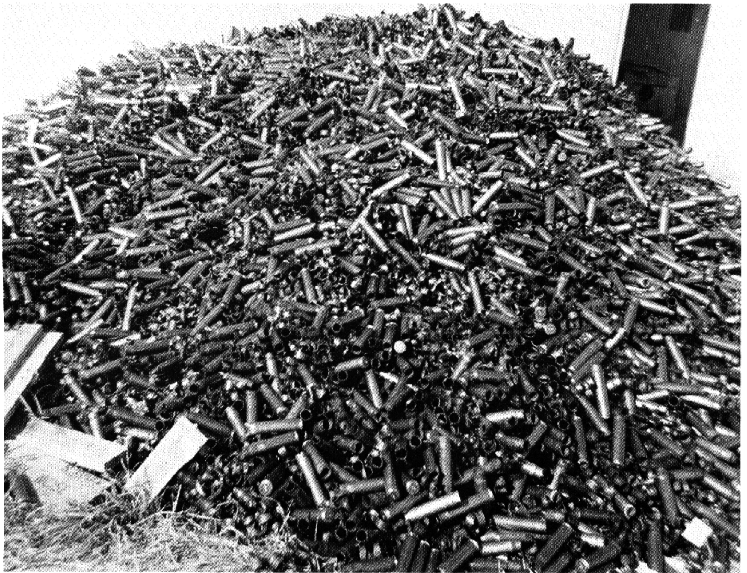
20mm Ammunition Fired During one Test using Chamber Lubricator and Ring Spring Mount.
