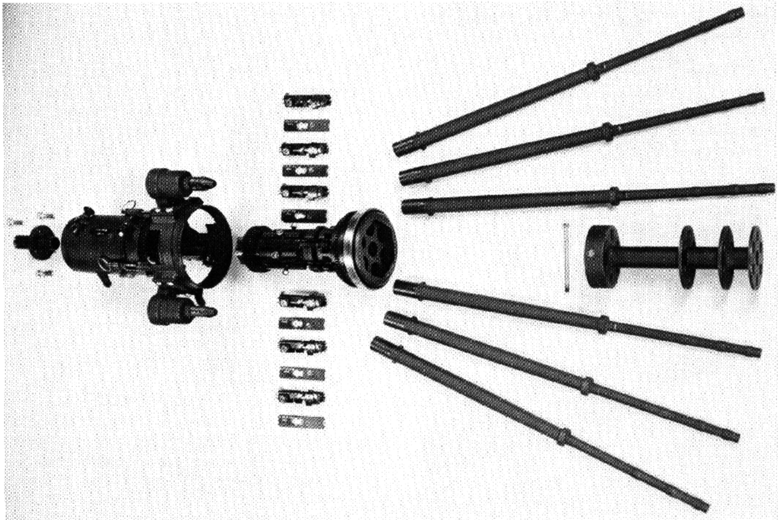
GAU-2B/A 7.62mm Aircraft Machine Gun Components
