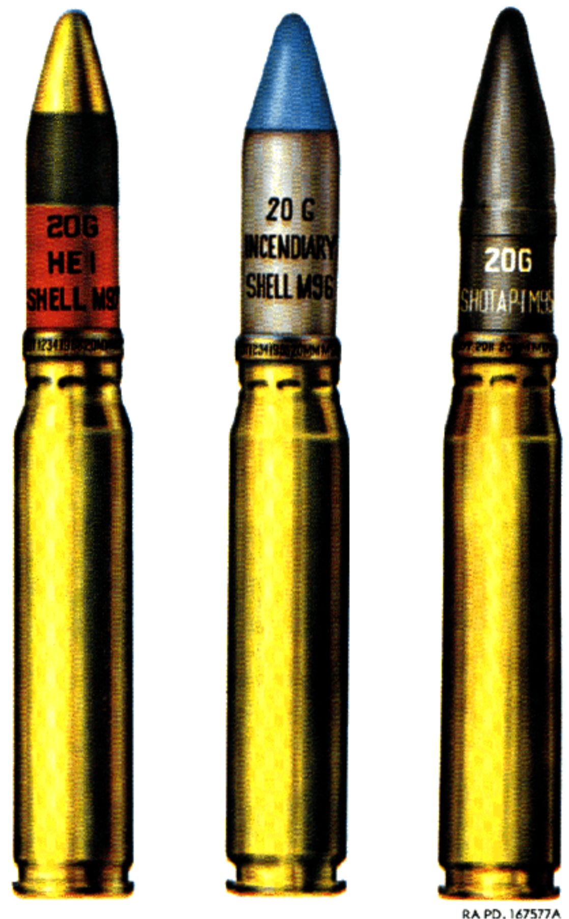
Color Identification and Typical Marking of Cartridges for Aircraft Cannon
