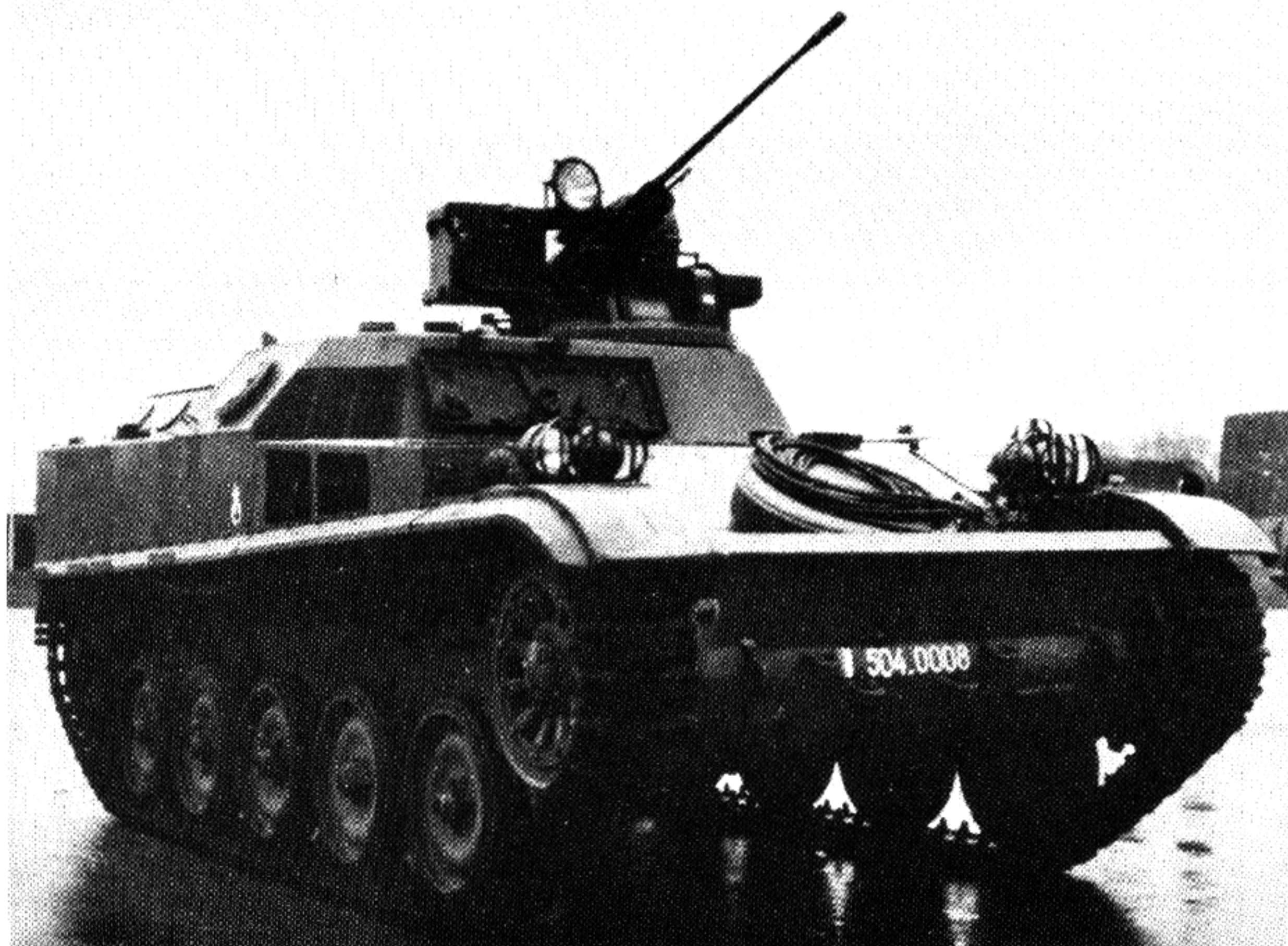
The M693 20mm Cannon is the Main Armament of the TOUCAN II Turret (TH 20) of the AMX 10 Infantry Combat Vehicle.
