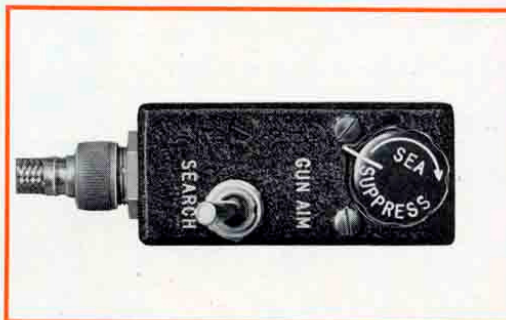
Figure 8—Auxiliary Control Unit
