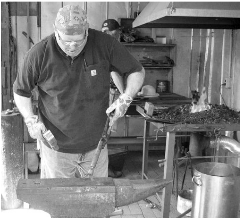
The author spreading the cut end of the pipe to form
