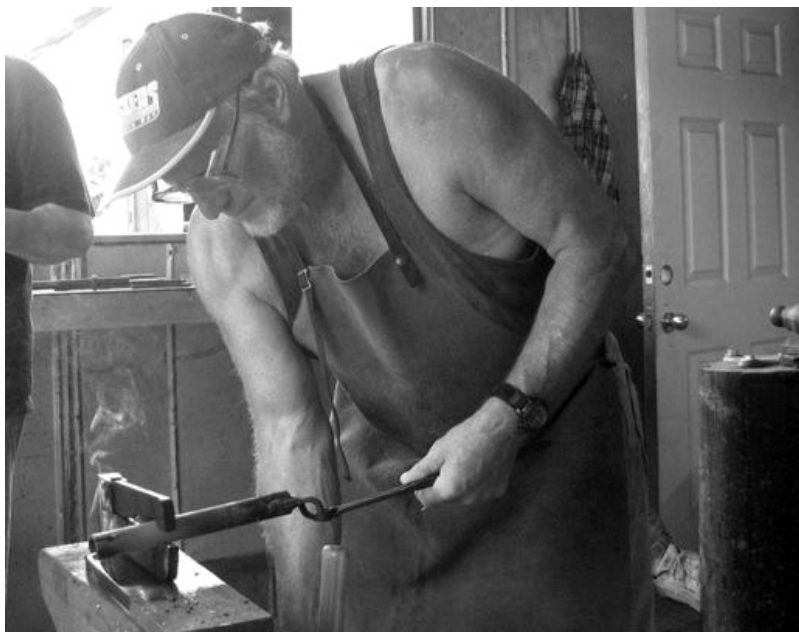
Allan Green using repaired fullering tool
