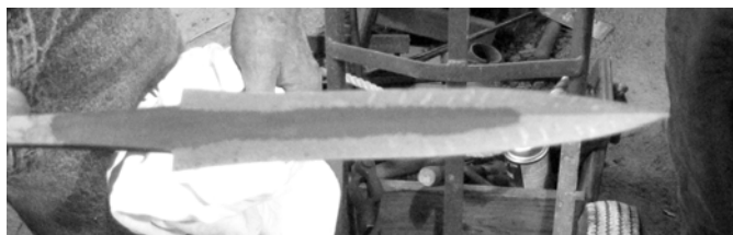
Blade Prepared With Refractory Material
