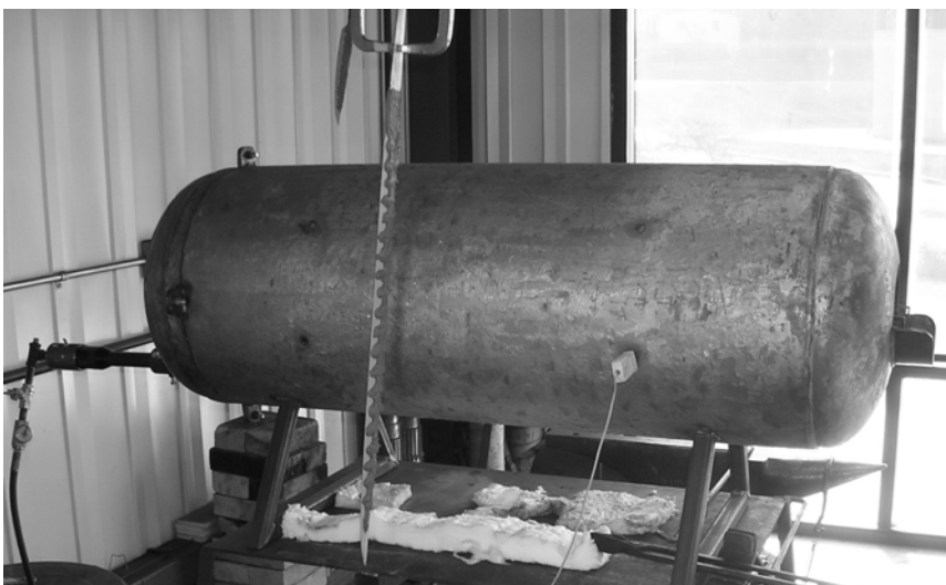
New England school heat treat furnace, made from salvaged propane tank. Note refractory coated sword blade hanging vertical left of tank center
