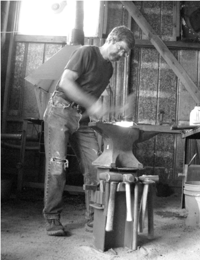
Robert Timberlake Forging a Knife Blade
