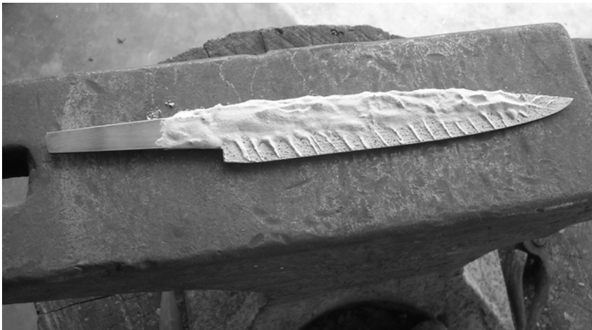
Refractory coated blade ready for heat treatment. Note ashi lines.
