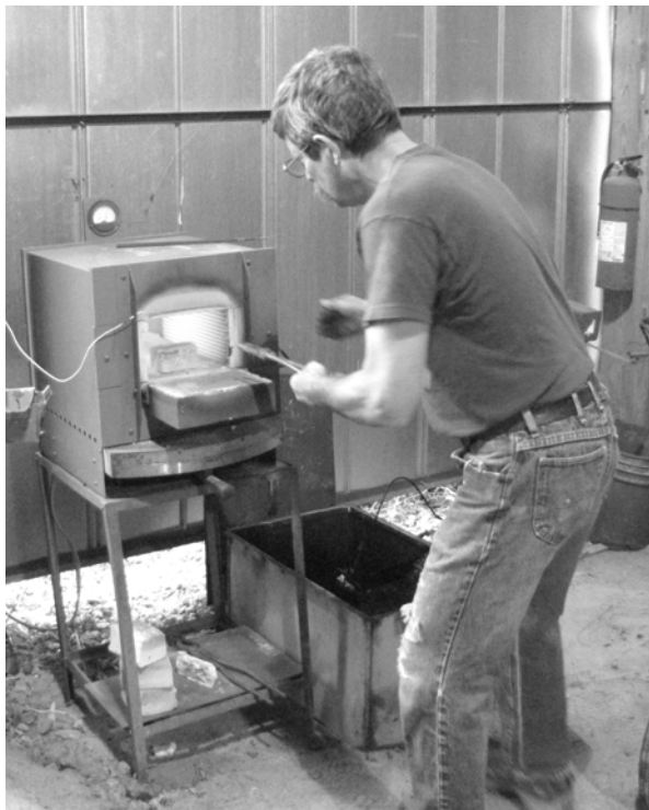
Heat-treatment In the Oven – Quench Tank Below
