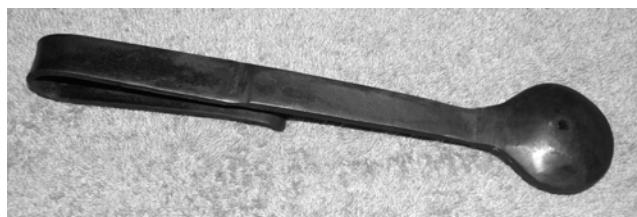
Close-up of a finished nail header.
