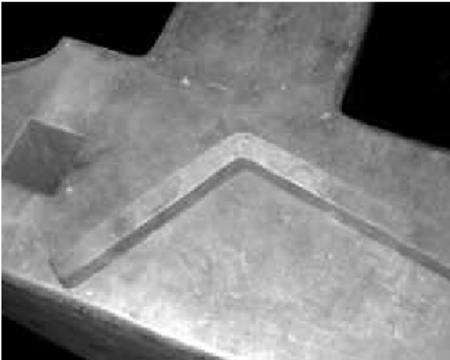
1. After the initial bend, the angle should be approximately 100 degrees, as shown here.
