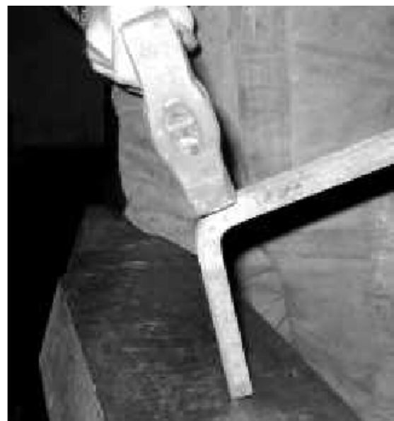
4. Vertical blow— note the position of the hammer and the short leg.
