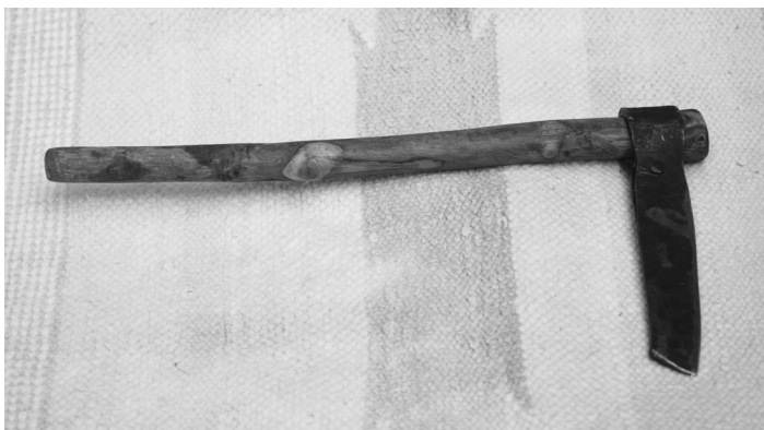
My very rustic froe – handle cut and shaved from a maple branch
