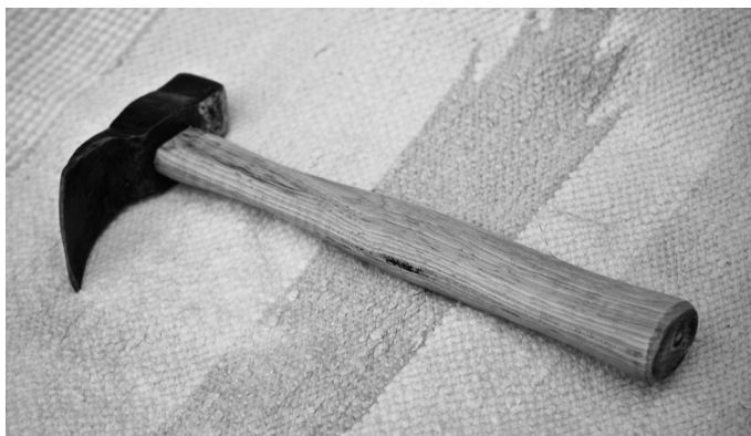
My bowl-hollowing adze—mild steel w/ tool steel cutting edge
