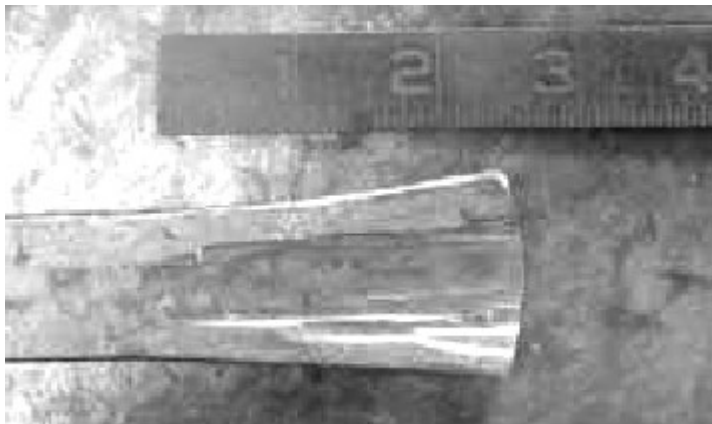
3. Centered trough formed by cross peen, 2 1/2" long.
