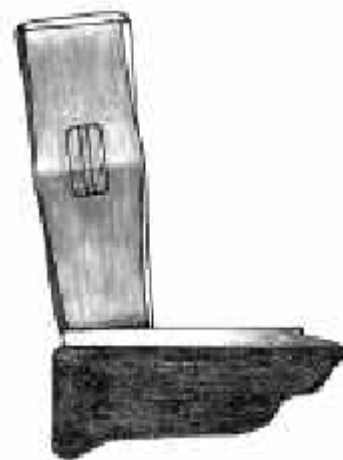
2a. The hammer head is tilted so the peen strikes the bar at the angle of the desired taper.
