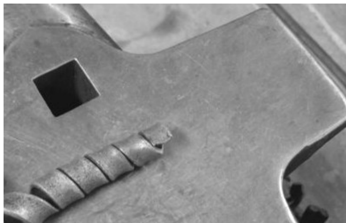
Continue rolling the bar until the desired amount of material is coiled.
