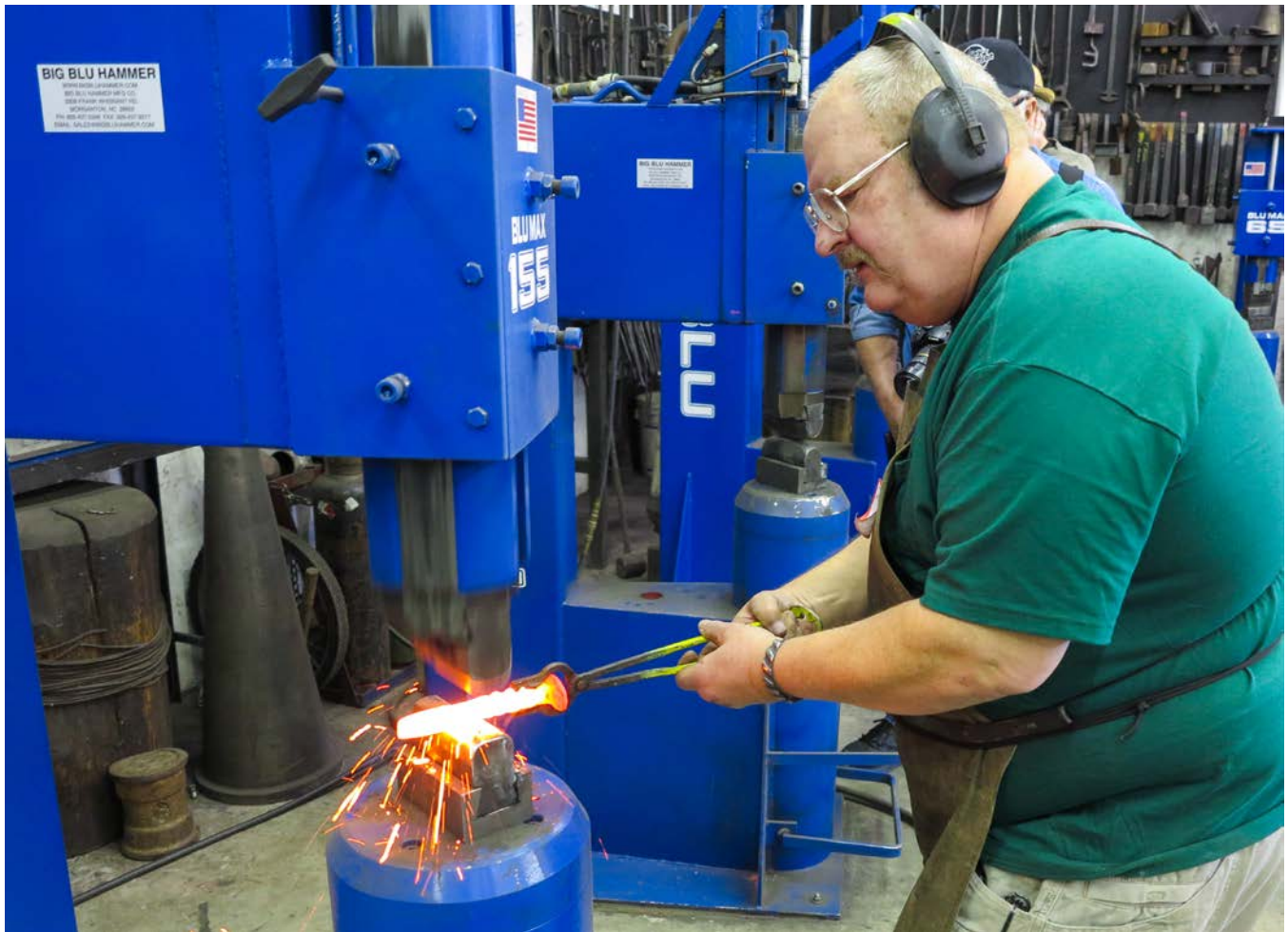
Doug Merkel forging a railroad spike knife at the NC ABANA quarterly meeting at Big Blu in Morganton
