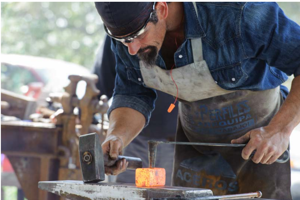
Brent Bailey setting the mark by hand before punching a hammer eye under the power hammer
