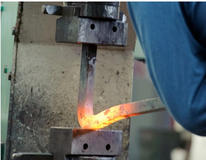
Forging an upset square corner under the power hammer
