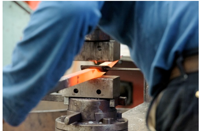
One end element is isolated from the stock
