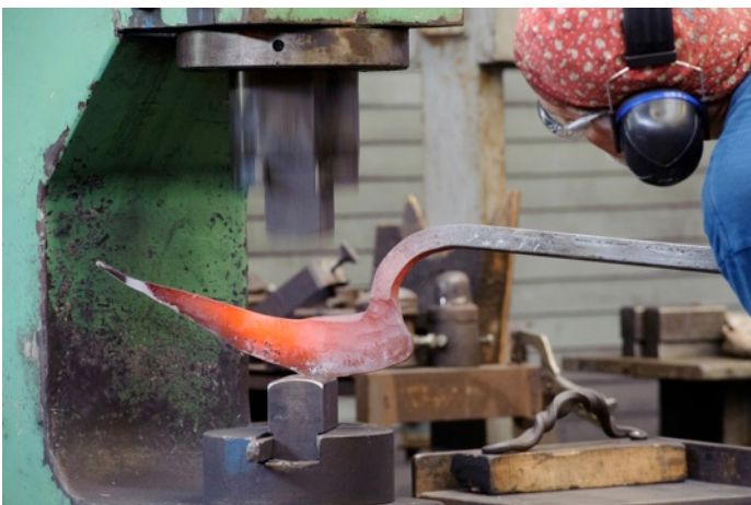
Refining a curve under drawing dies
