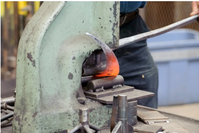
Bending a smooth curve under the flypress
