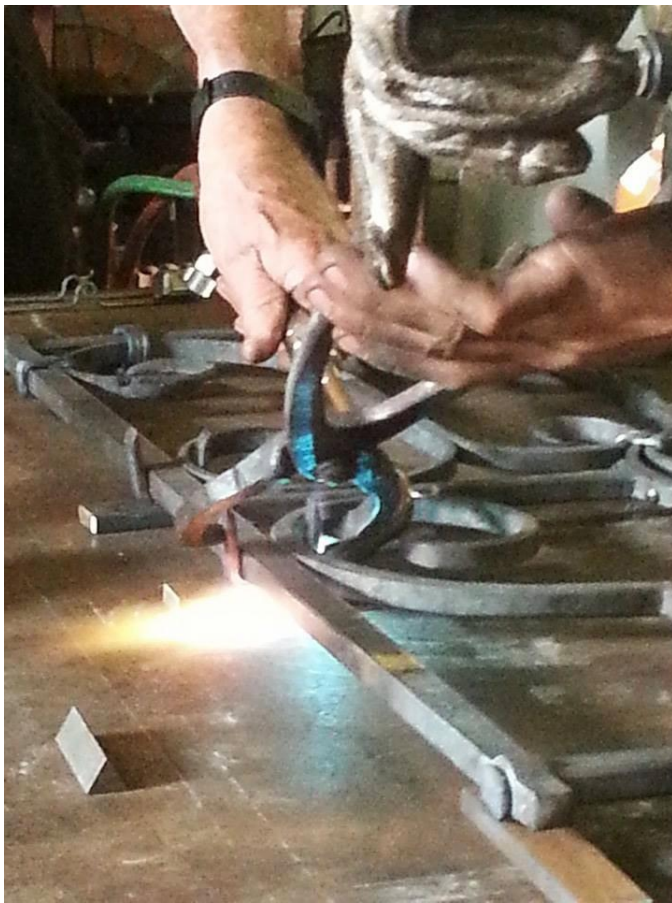
Collar detail of the window grille
