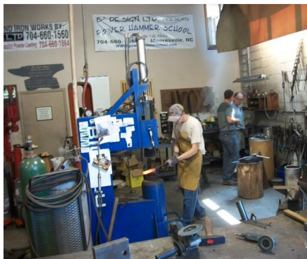
Big Blu power hammers work large stock
