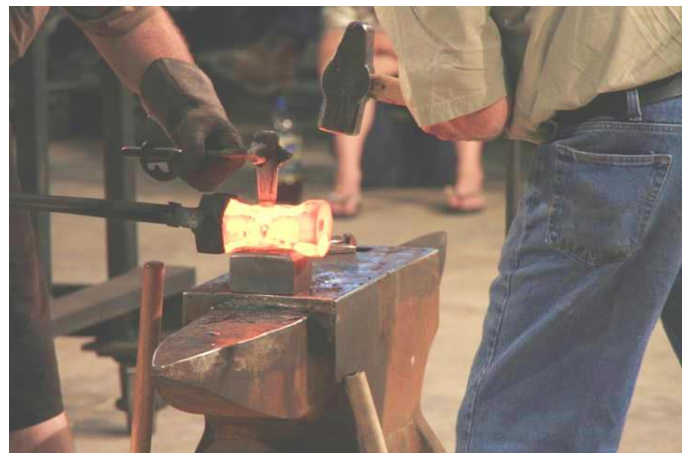
Punching an eye in a Damascus hammer on 1000lb anvil
