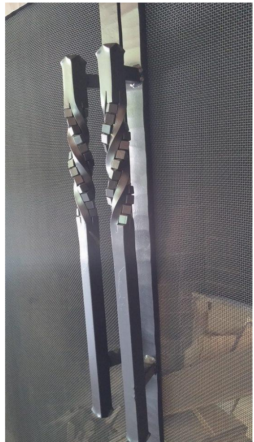
These are the detailed handles for the fireplace screen above. I know many smiths will appreciate the complicated twist that went into them.
