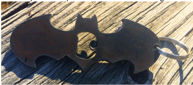
Next is Iron Mountain's top seller: batman bottle openers. While the shape is cut using a plasma table, the opener part in the center has to be forged to function.
