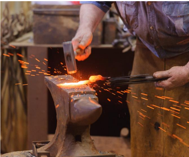
Stick the weld; speed to the anvil and a light touch as needed.
