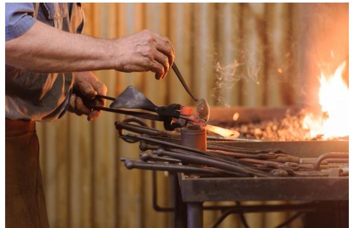
Heat and flux while still keeping the pieces in position in the tongs.
