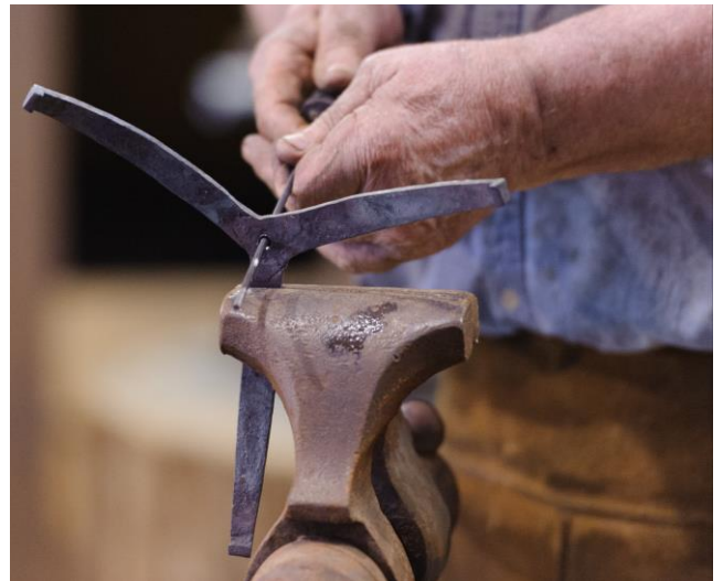
Adjusting the hole in base to fit the tenon.
