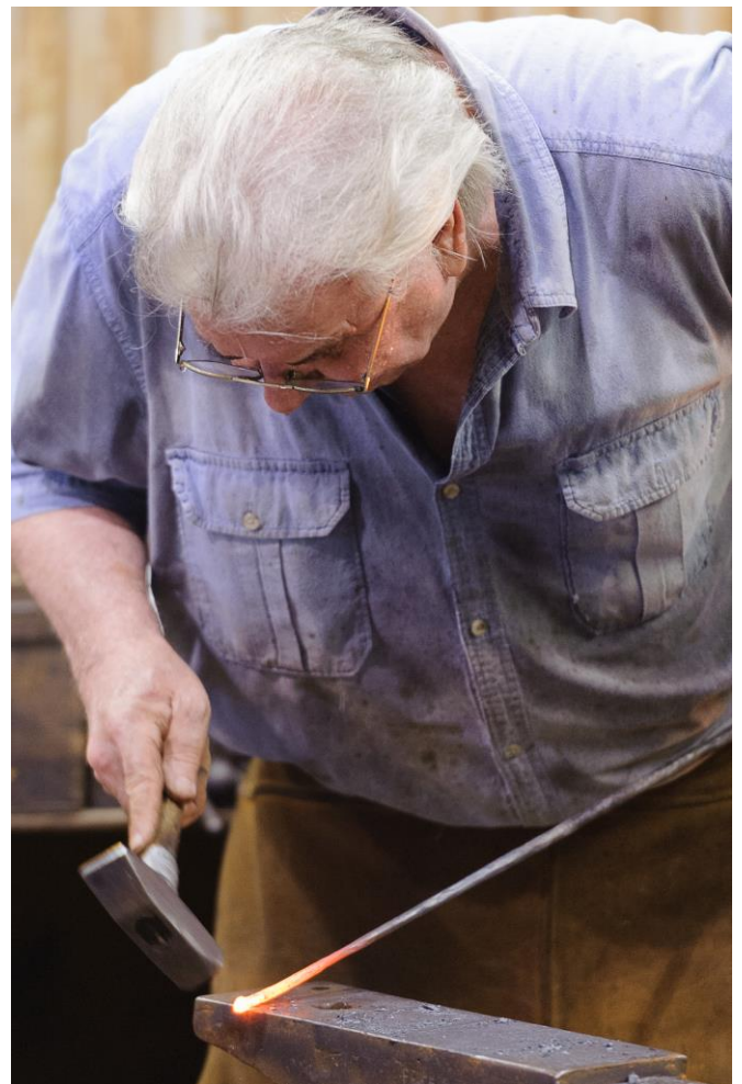
A small mass is left after tapering the top end of the upright and a small ball is forged on the end. Here Jerry uses the edge of the anvil as a backup to help forge the ball.
