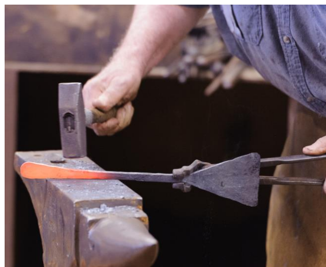
Round the end and smooth the taper into the forge weld.
