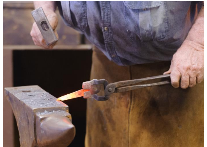
Scarf the tongue for a Jump weld.
