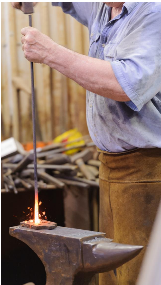
He uses a plate with holes as a monkey tool to square up the shoulder of the tenon.
