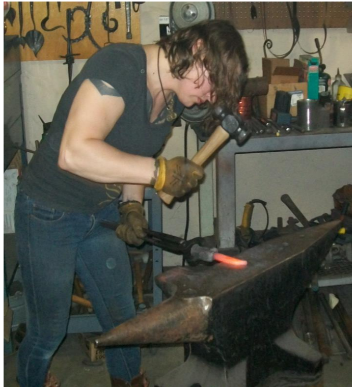
Avery Pierce hand forging a railroad spike knife
