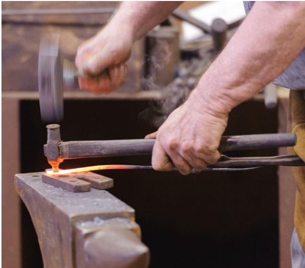
Widen the hole to size with the back end of the punch.
