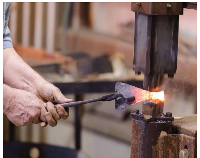
Forge the cone blank stem down to 5/16" in preparation for forge welding the slide.
