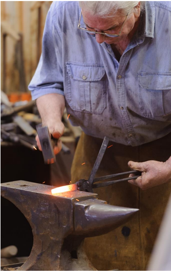
Taper the ends and chamfer the sides
