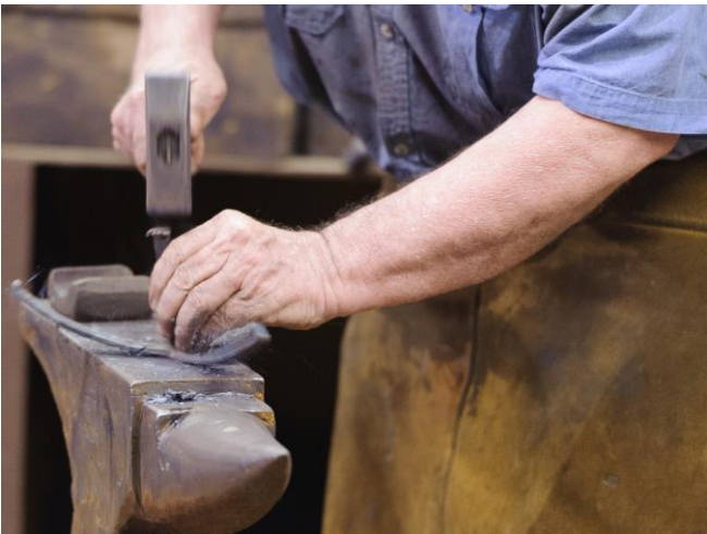
Jerry center-punched the base, and had a ¼" hole drilled and countersunk on the bottom for riveting a flush tenon.
