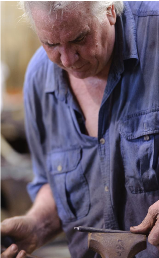
Cleaning the tenon on the upright with a file
