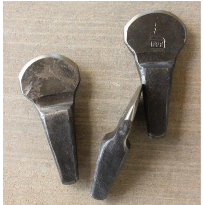
These Hardy tools were also made with 4140. The sharp edge for cutting mild steel makes 4140a great option for hot cuts.
