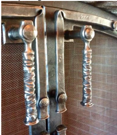
It is not just the original texture on the handles that is impressive but also the large rivets and folded corners.
