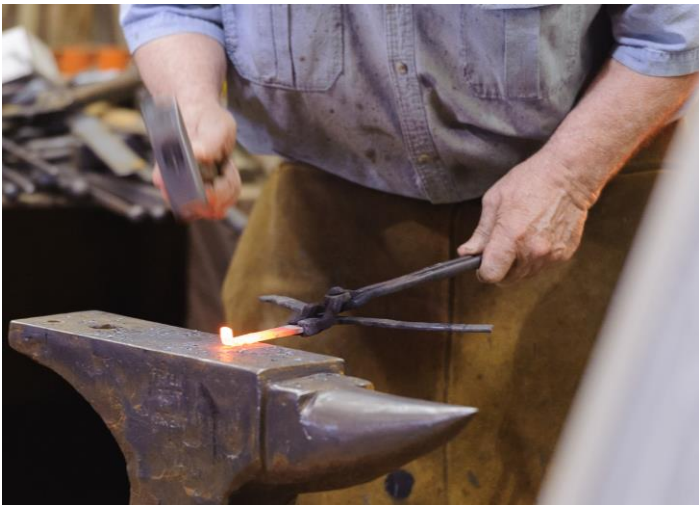
Turn the feet \sim\frac{3}{4} " and upset to \sim\frac{1}{4} " thick
