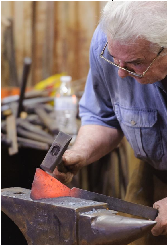
Applying the final touches to the cone form.
