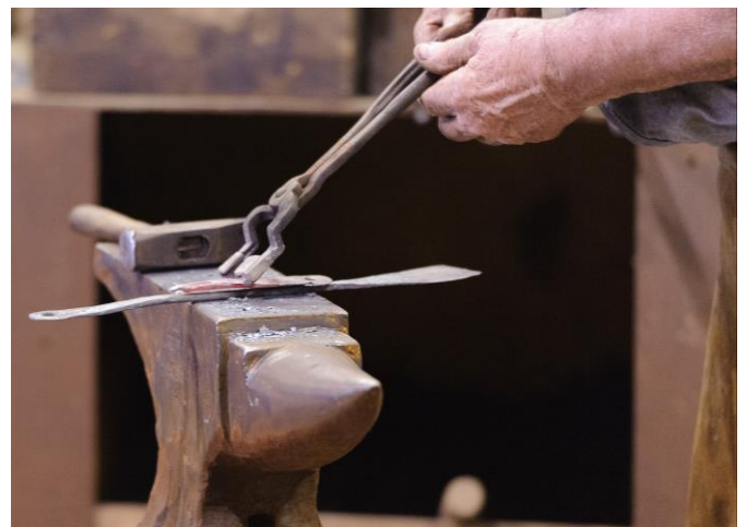
Align the tongue on the cone form and grasp in the tongs in preparation for the jump weld.
