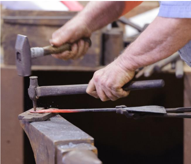
Punch through over a hole in a backing plate
