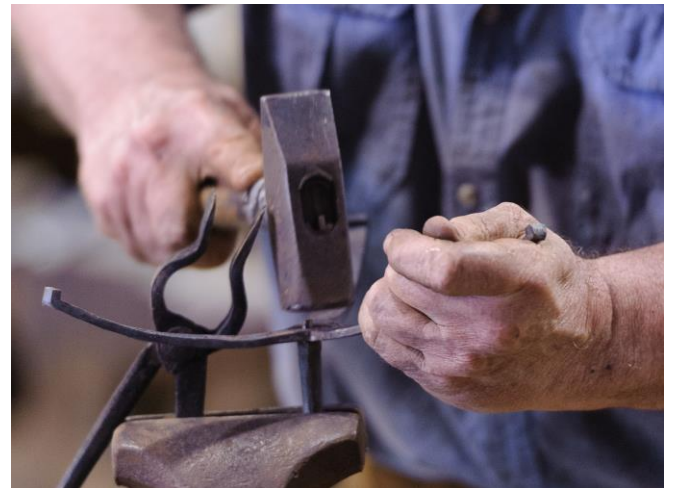
Setting the tenon to fasten the base to the tenon.
