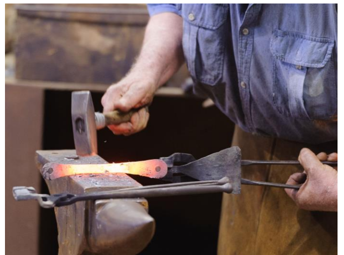
The result should be a smooth tapered connection of the tongues.
