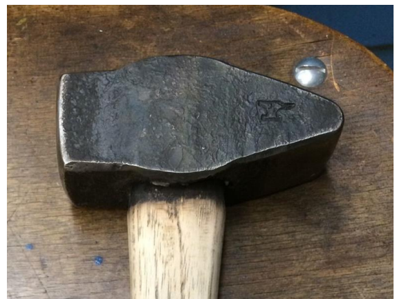
This Hofi style hammer head was made with 4140. It is also great for other things that go on the end of a handle like tomahawks and axes.
