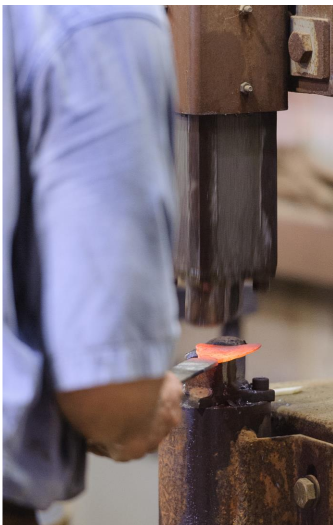
The form for the cone is then spread on drawing dies on the power hammer.
