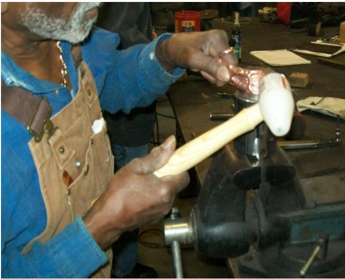
The vice is an important tool to utilize when folding copper
