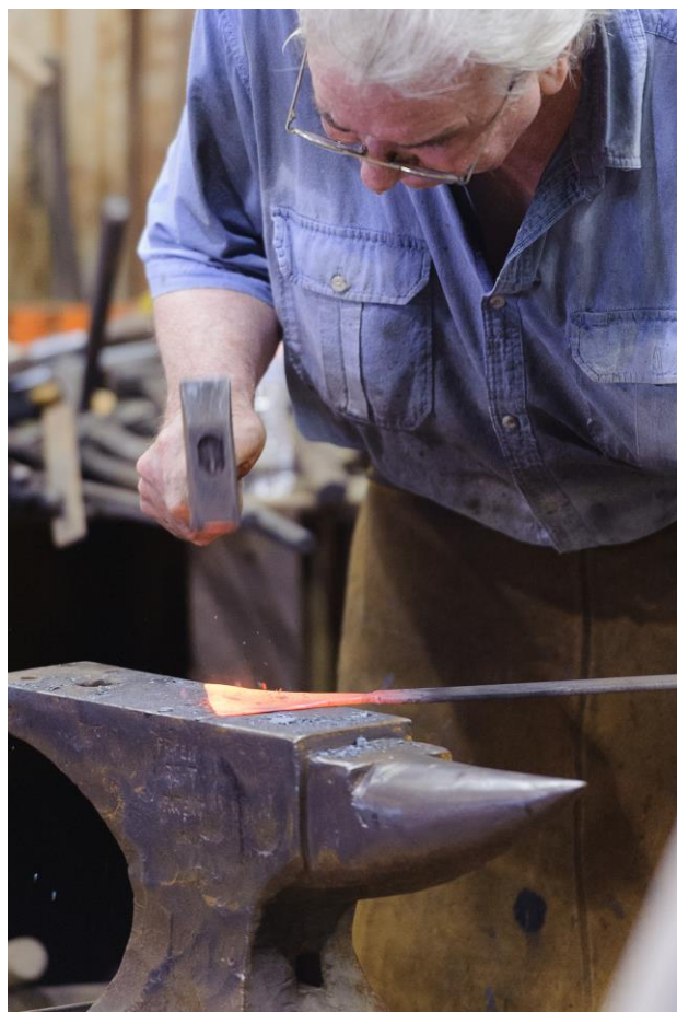
The blank is evened out and refined on the anvil.
