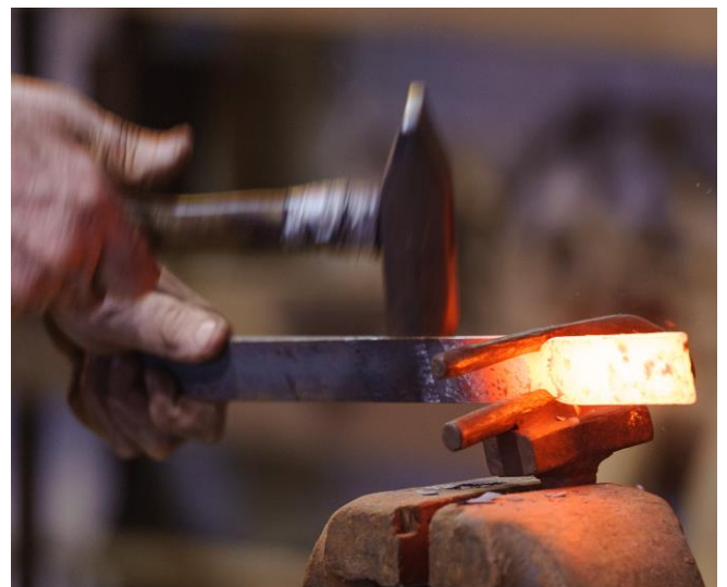
To start forging the candle cone, about 3" is isolated on the end of a 3/16" x 1 ½" bar.
