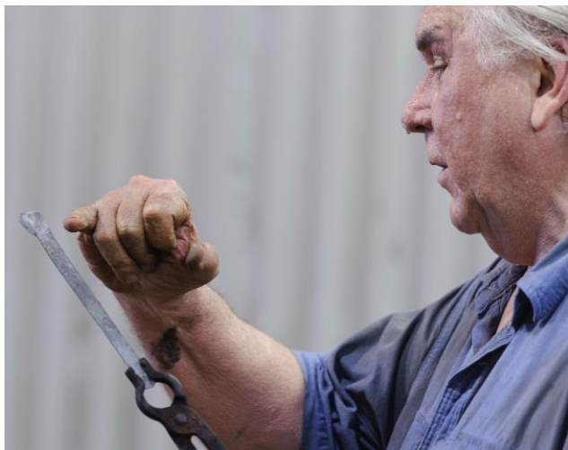
Forge a tongue on each end and shape the spring to a pleasing taper.
