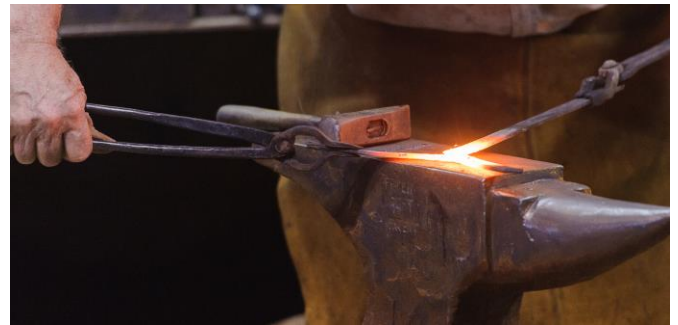
Setting up the two scarfed pieces for a drop-the-tongs weld of the tripod base
