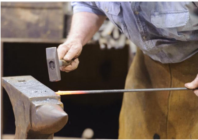
Jerry's great hammer control was demonstrated in hand forging a ¼" tenon on the upset stem of the upright
