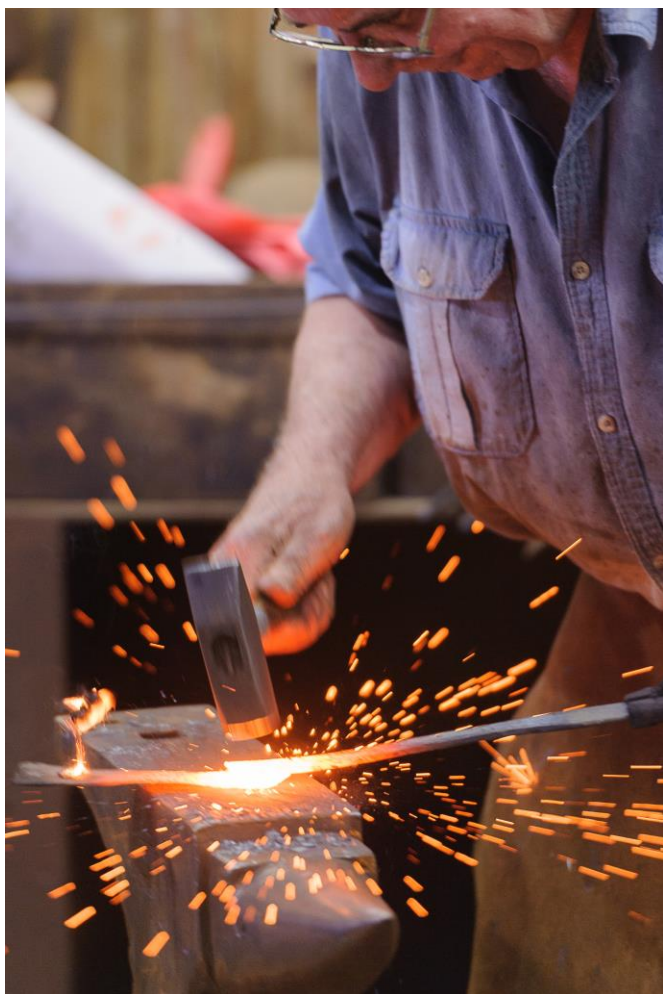
Forge weld the cone form to an 8" piece of 3/16"x3/4" tapered to 5/16" and scarfed.
