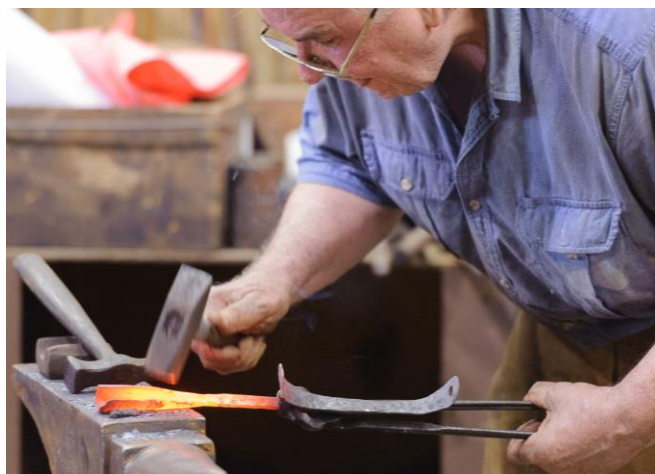
Close and even the cone with light hammer work on the anvil.
