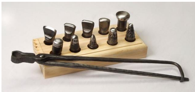
Pictured above is a good-sized fullering tool set complete with tongs for holding the tools. Pictured below is the ball fuller.
