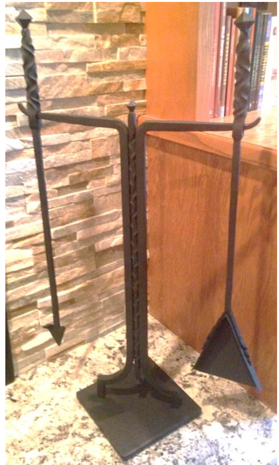
This picture above shows just how much time went into the fireplace tools and holder. Note the long twist along the centerline of the stand. Below is a better detail of the shovel's flare and riveted ends.
