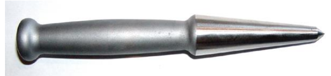
Center punch tool created with 4140. Punches one of the best uses for this steel.
