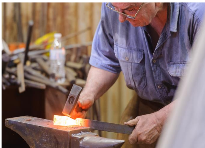
The bottom end of the cone is tapered on the anvil.
