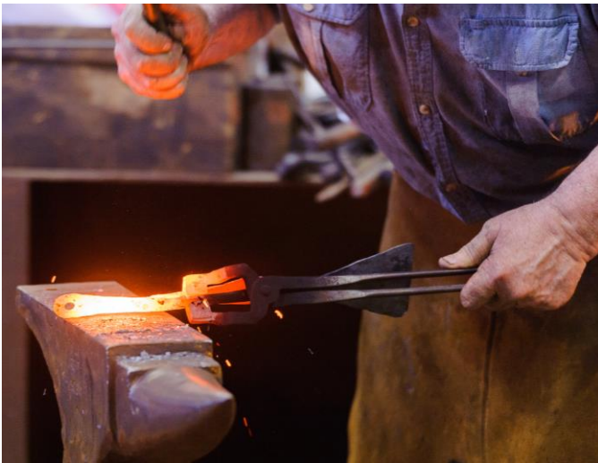
Stick the weld; speed to the anvil and a light touch as needed.
