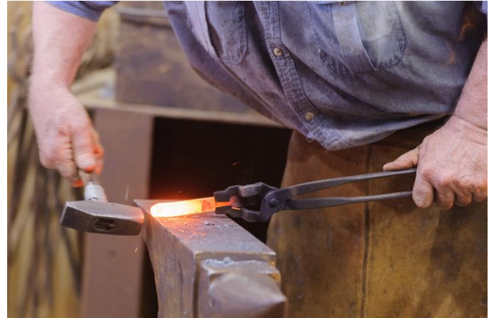
Forge a tongue from 5" of 3/16" x 3/4" stock starting by rounding the end
