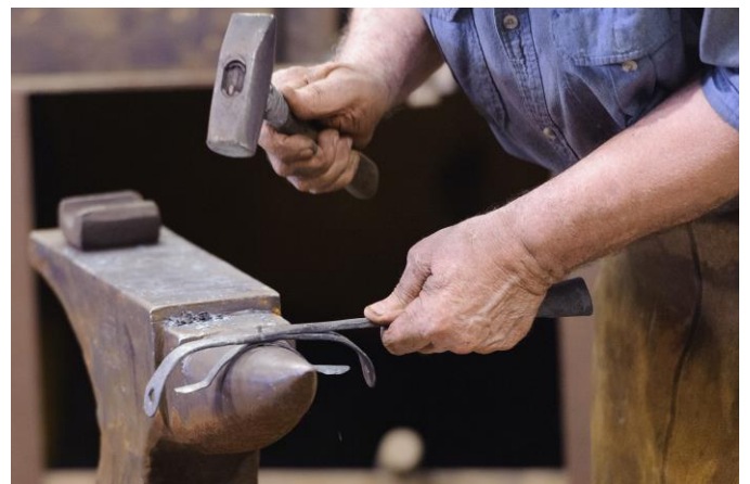
The spring and candle holder have been drilled and Jerry is setting an eighth inch rivet to hold them together.
