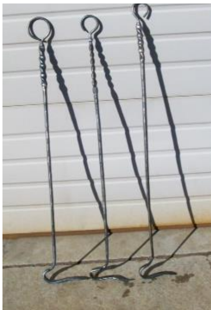
3 firepokers forged by Tyler Rasche under a Big Blu power hammer
