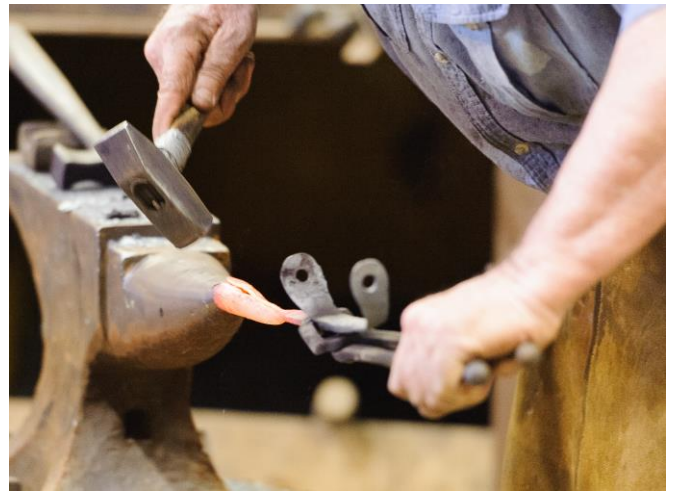
Even and straighten the cone on the horn.
