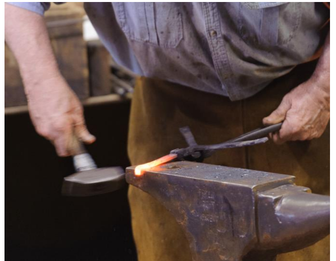
Finish the feet up as you would an upset corner
