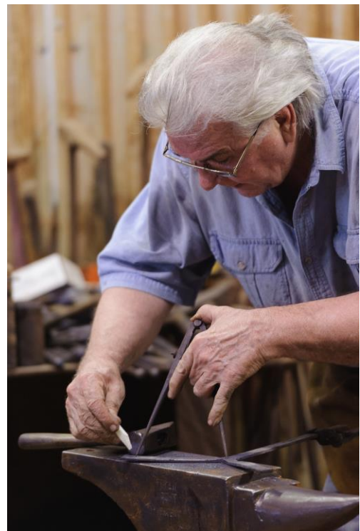
Jerry uses dividers to mark for cutting all the legs to 5"
