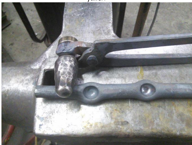
Pictured above is a good-sized fullering tool set complete with tongs for holding the tools. Pictured below is the ball fuller.
