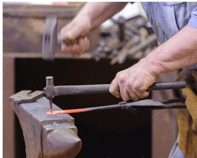
Start punching the end for the 1/4" upright.
