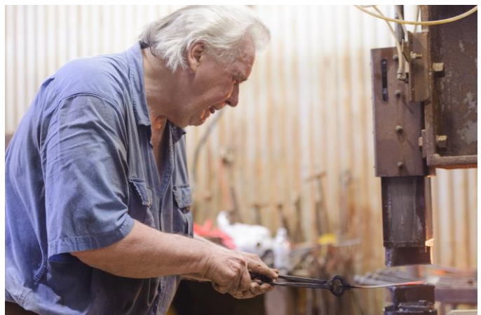
Forge the spring from 3/16" spring stock. Here Jerry is flattening 6" of stock to ~1/2" under the power hammer.
