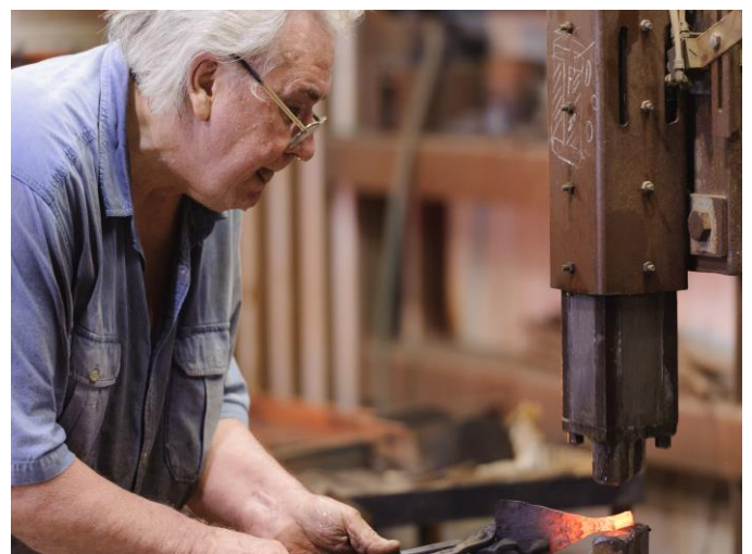
Ready to scarf for the forge weld.
