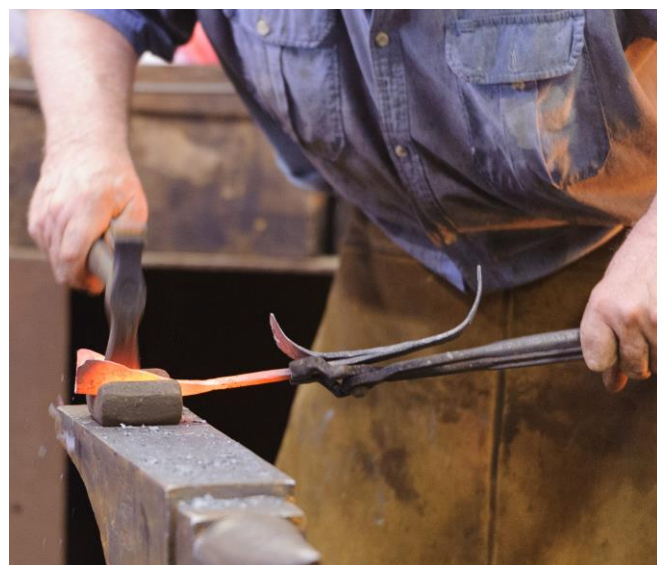
Roll the candle cone in a swage.
