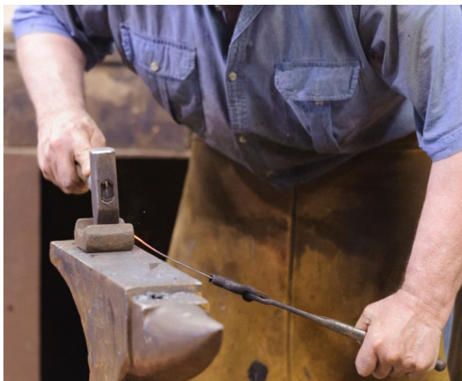
The ends are then curved in a swage.
