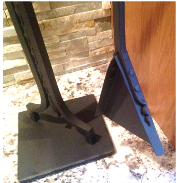
This picture above shows just how much time went into the fireplace tools and holder. Note the long twist along the centerline of the stand. Below is a better detail of the shovel's flare and riveted ends.
