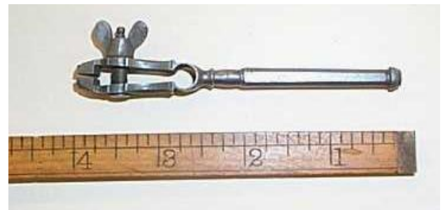
Note the true size of a pin vise in the above picture.
