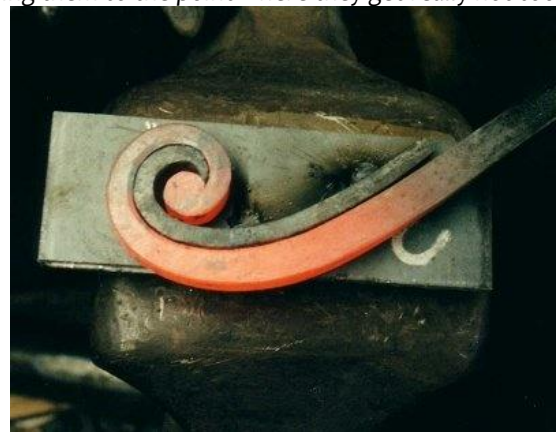
Whether your jigs look like the picture above or below, 8620 is a great steel to build them with if you are going to be using them to the point where they get really hot too.
