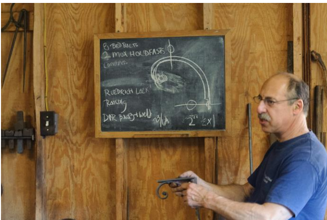
Peter discusses the sequence to fit a scroll to a bracket using rivets
