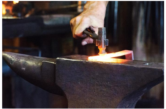
Countersinking the bracket back for a flush rivet
